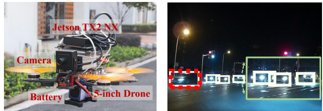
(a) Implementation of Anole on Jetson TX2 NX deployed on a UAV. (b) Results in a typical night scenario.
