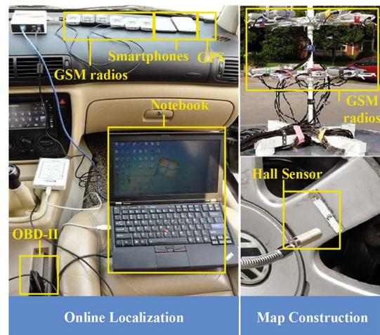
**Fig. 11** Our prototype implementation of UPS
