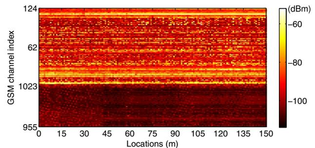
**Fig. 1** Illustration of GSM power spectrogram of 194 channels collected over 150 m
