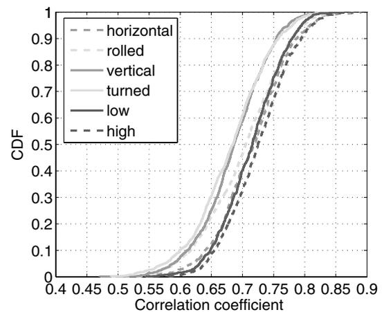
**Fig. 10** Similarity between different GSM radios with different placements
