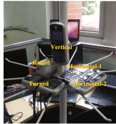
**Fig. 9** GSM radios set in different orientations
