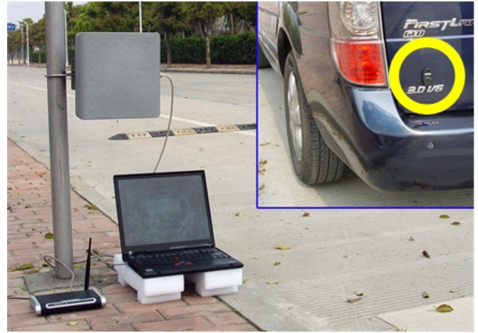
Fig. 11. Local node with an RFID reader and a wireless AP. The highlighted area in the inset shows an active RFID tag attached to a vehicle.
