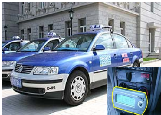
Fig. 1. A taxi with a commercial GPS device installed, the highlight area in the inset shows a device consisting of a commercial GPS receiver and a GPRS wireless communication module.
