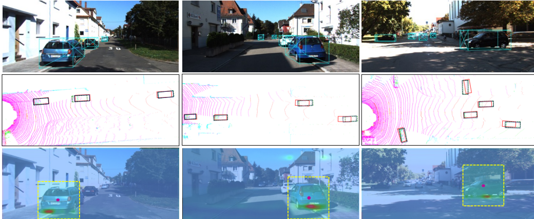
Figure 5: Qualitative results on KITTI Odometry dataset. The predicted 3D bounding boxes of our proposed MoGDE are shown in the first row. The second row shows the detection results in the bird’s eye view ( z -direction from right to left). The green dashed boxes are the ground truth, and the blue and red solid boxes are the prediction results of our MoGDE and the comparison baseline (GUPNet [27]), respectively. The third row visualizes the results of the attention map in transformer’s encoder, where the purple point is the location of the query point; the yellow dashed box is the range of encoder’s mask; and the brightness of the image represents the attention value between the query point and that pixel.
